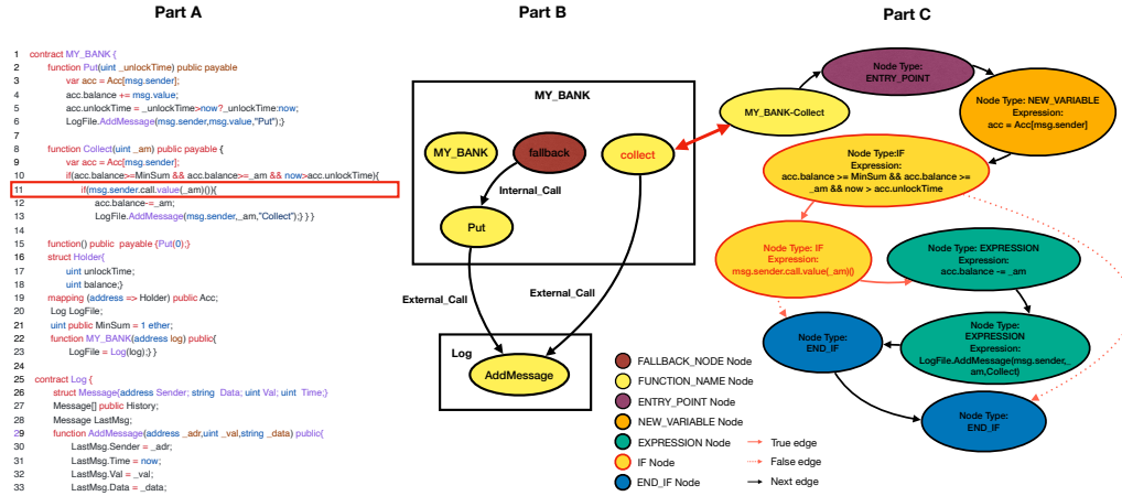
FIGURE 6.1: A sample Ethereum smart contract MY_BANK (Part A), its call graph (CG) (Part B), and a control-flow graph (CFG) (Part C) for the function Collect. Line 11 in Part A is the root cause of a reentrancy bug; the nodes in CG and CFG containing the reentrancy bug are highlighted with red text.
